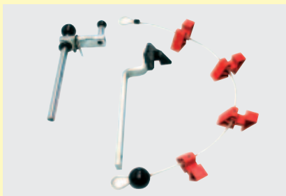
G800A15 Premitalлоне 22". 22" bead pushing device. Wulstboy 22".
