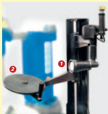
Dispositivo premialza tallone pneumatico. Air-driven device for bead pushing-raising. Pneumatischer Hilfsmontagearm.
