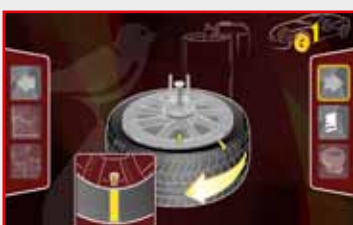
Match-Mounting procedure (rim-tyre)
