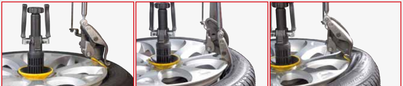
Top bead demounting procedure
